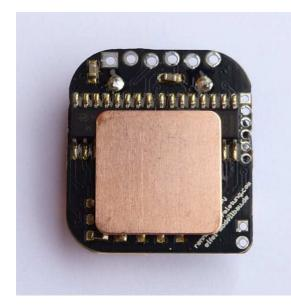
Without a cooler the SLC will work up to the following loads as a function of the input voltage: 6 Volts – 400 mA, 12 Volts – 150 mA, 18 Volts – 100 mA \*. Please note that without any connected
