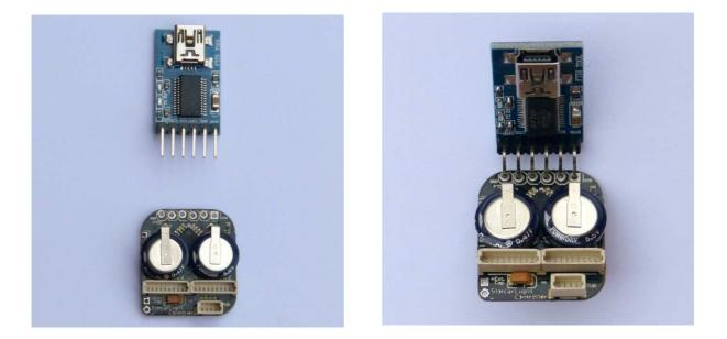
To reprogram the SLC with the SLC Manager the USB-FTDI adapter has to be connected as seen in the pictures. After choosing the COM-Port in the SLC Manager, the upload can be started with the upload button.
