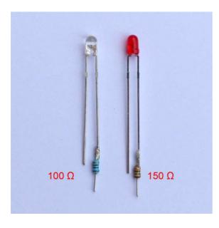
The pluspin of the output connector has to be connected to the anode (the long leg) of each LED. The channels 1 to 14 depending on their function have to be connected to the cathode (the short leg) of the LED, each with a fitting resistor.
